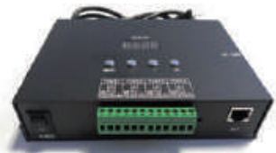
H806SA Can be connected to the DMX console, can be used for online point tracing, and multiple controllers can be powered on simultaneously to achieve synchronization among multiple controllers.
